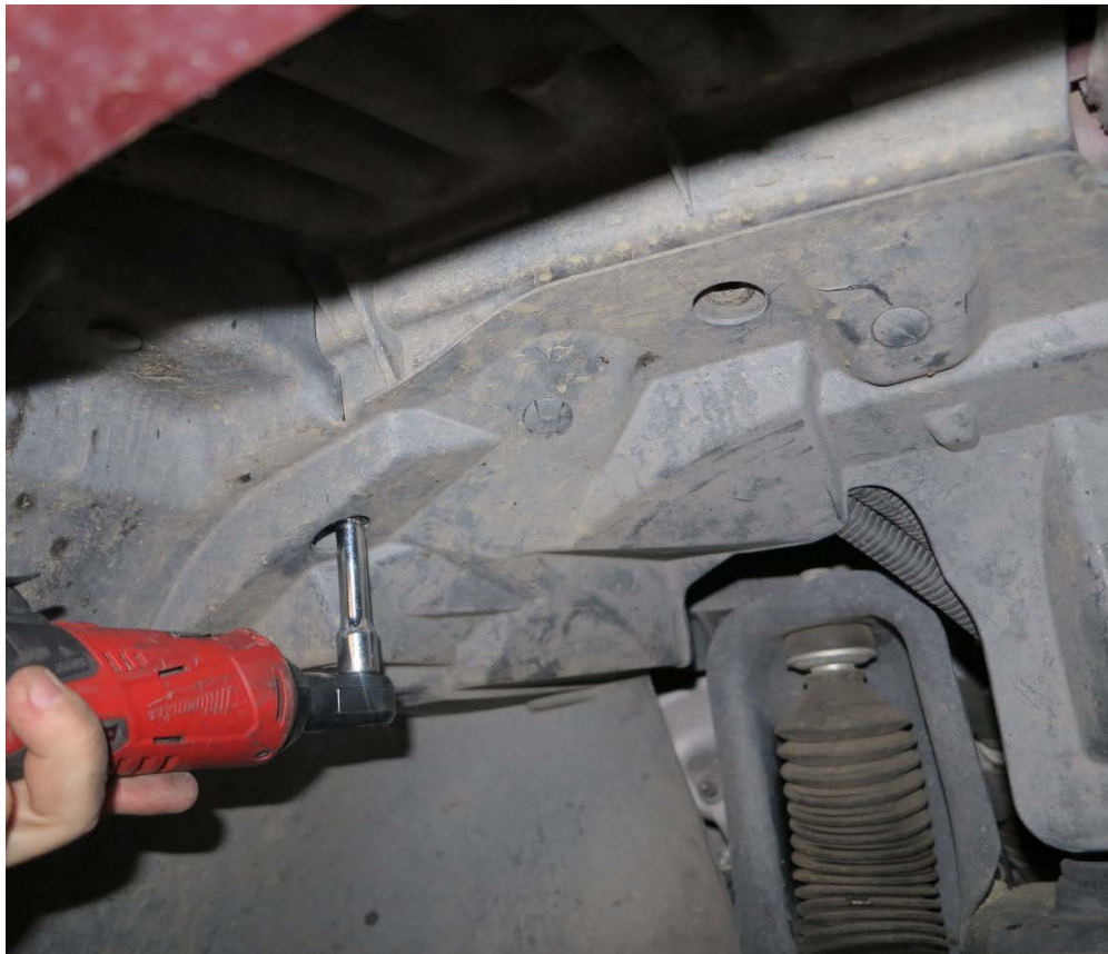
(Figure 6) Remove the 6 bolts securing factory fender liner.
