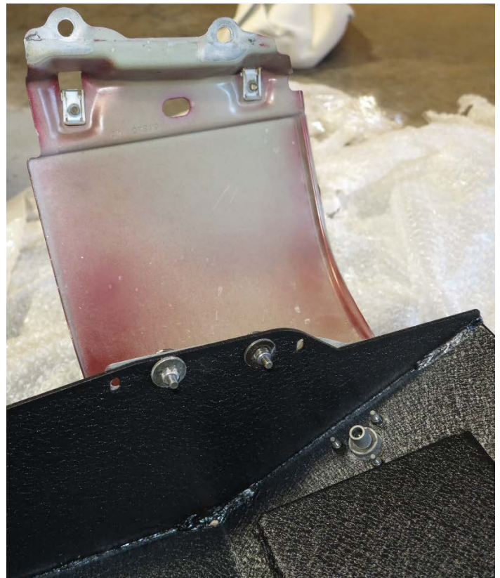
(Figure 16) Attach the side cowl to the fender using (2) 6mm x 25mm Hex Bolts, (4) 6mm x 12mm Flat Washers, and (2) 6mm Nylon Lock Nuts.
