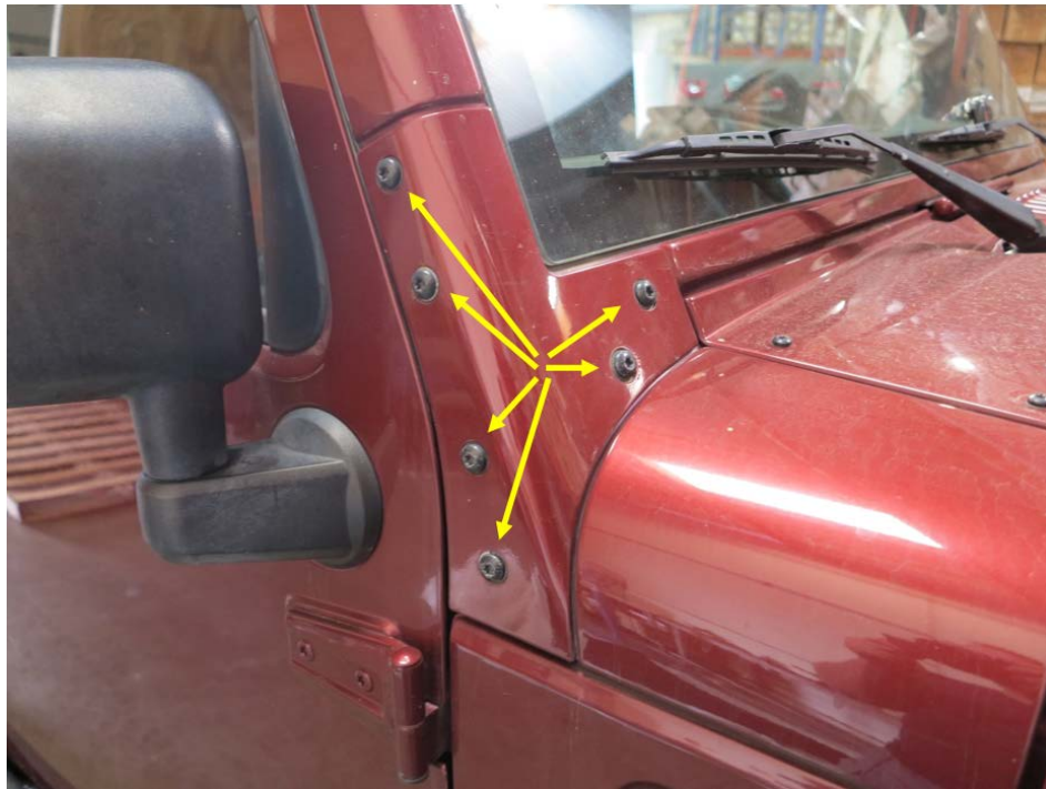
(Figure 2) Remove bolts to free windshield bracket.
