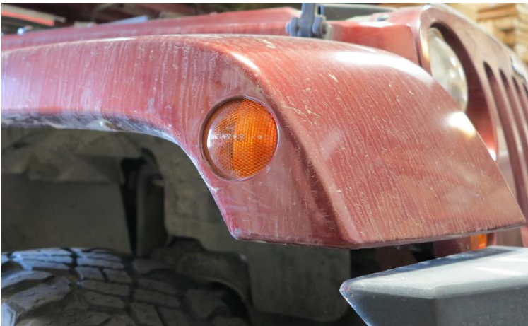
(Figure 9) Unplug side marker wiring and unclip wiring from fender.
