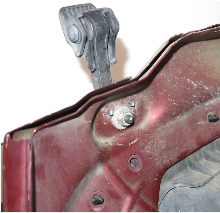
(Figure 14) Transfer hood latch to your new RBP fender reusing the factory nut.
