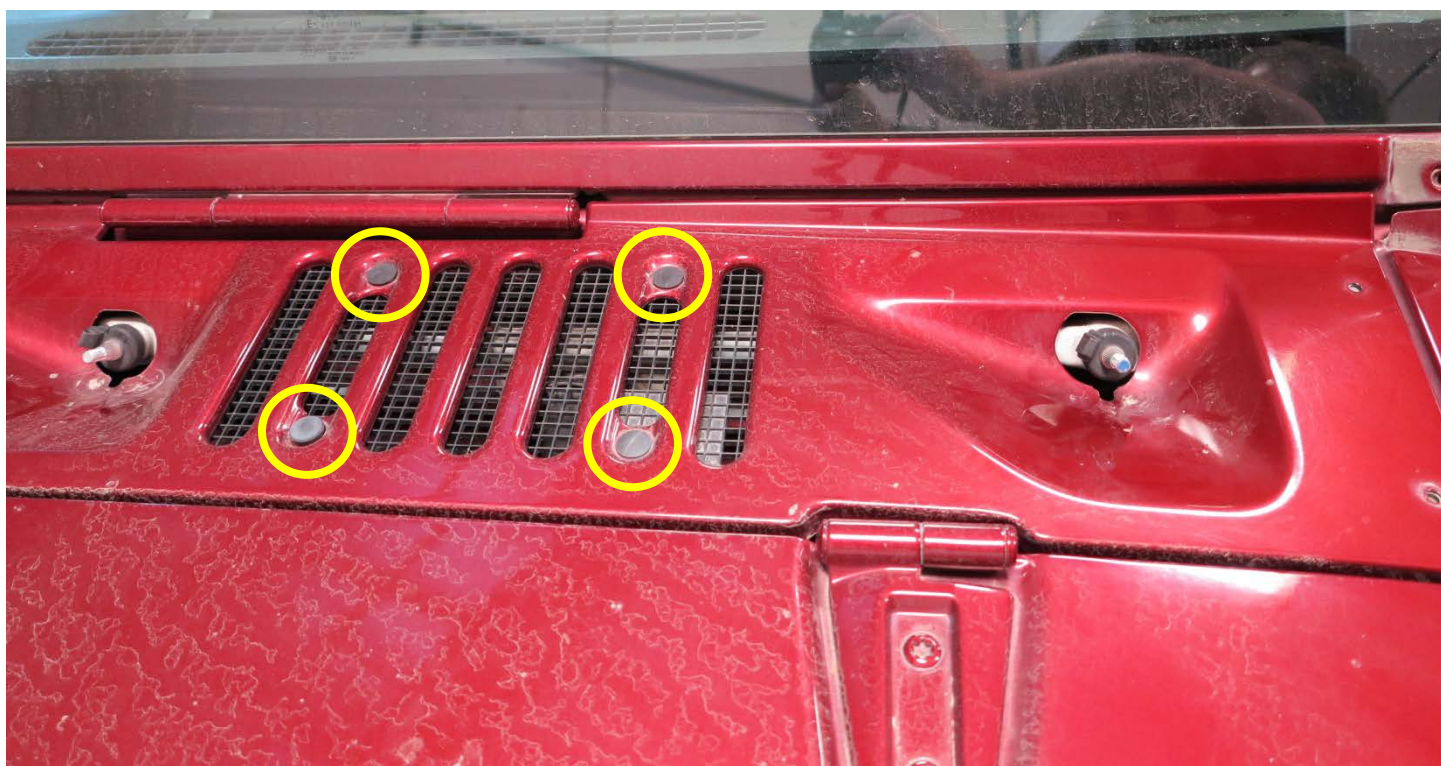
(Figure 4) Remove the 4 plastic clips and gently set aside the cowl for reuse.
