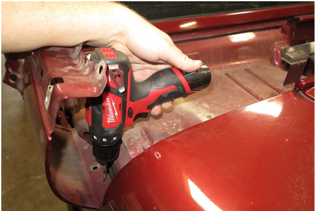
(Figure 5) Drill out spot welds with 1/4" drill bit.
