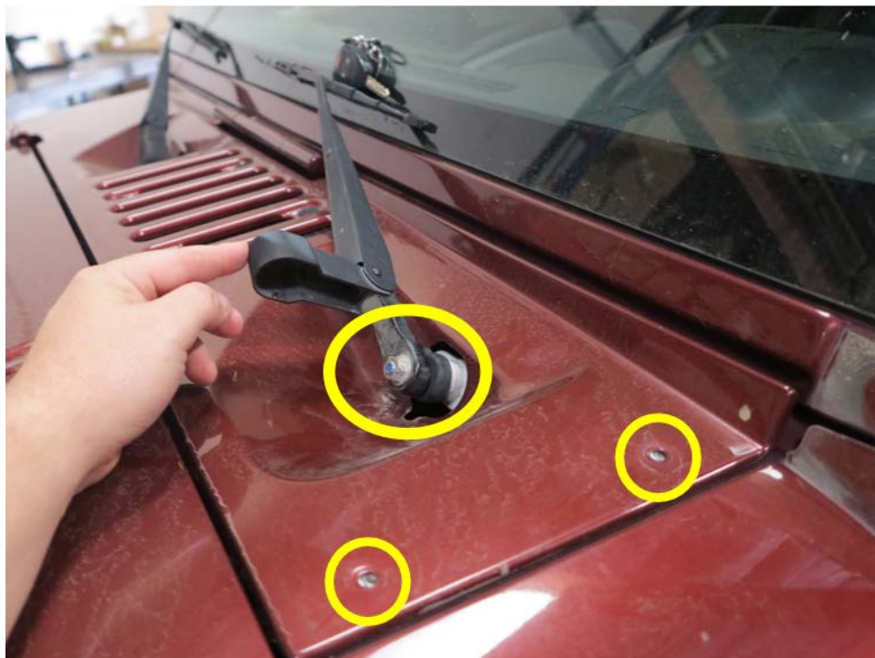
(Figure 3) Lift up the plastic covers and remove nuts at the base of the windshield wipers. After the wipers are free, remove the 2 bolts on each side of the cowl.
