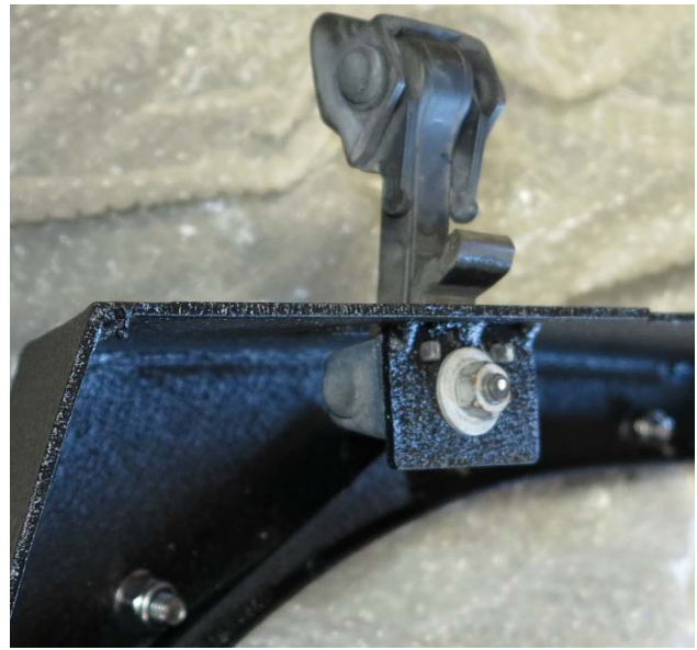
(Figure 14) Transfer hood latch to your new RBP fender reusing the factory nut.
