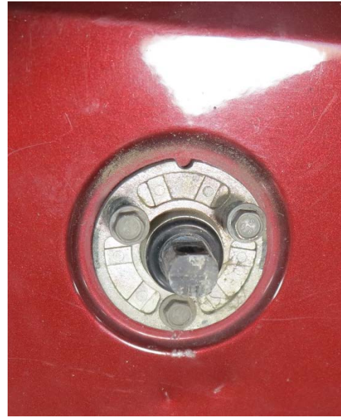
(Figure 8) Remove the 3 bolts and unplug antenna wiring.
